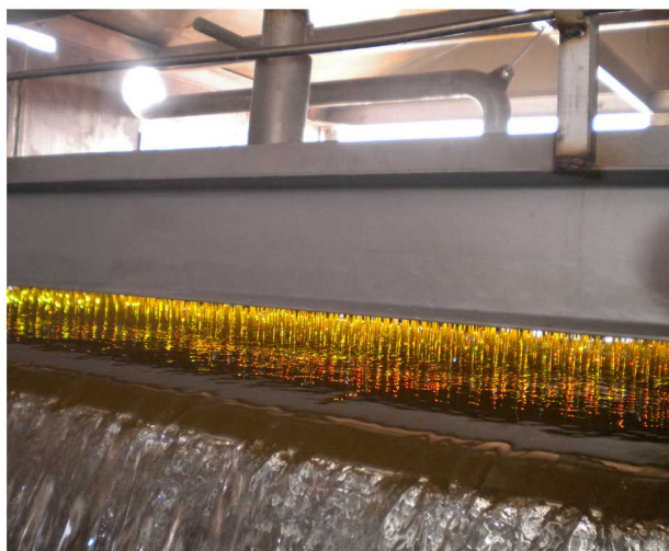
Figure 3. Molten sulfur at forming tray above the water column.
