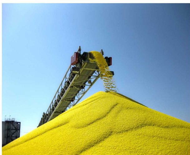
Figure 4. No airborne dust as sulfur prills are stockpiled.
